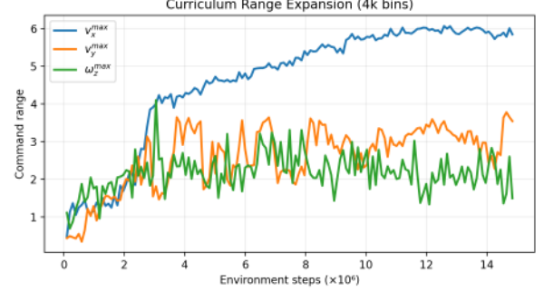
Fig. 3: Curriculum range expansion over command space: TransCurriculum expands the initial command range of [-1.0, 1.0] in increments of \pm 0.5 based on stable velocity tracking. The maximum sampled commands, v_x^{\max} , v_y^{\max} , and \omega_z^{\max} , show that the forward-speed range expands steadily, whereas the lateral and yaw-rate ranges saturate at lower values, consistent with the forward-locomotion reward design. Actual environment-step counts are ten times the displayed x-axis values.
